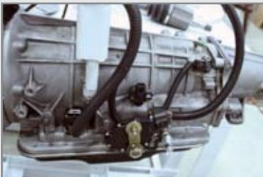
The MAE-TCM gives you the ability to test a transmission using the correct frequency and duty cycle, which ensures that the transmissions are being tested exactly as they perform in a vehicle.
