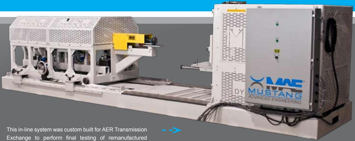
This in-line system was custom built for AER Transmission Exchange to perform final testing of remanufactured transmissions. The system has a variable speed AC dyne motor and a dual eddy current PAU output loading dyne.
