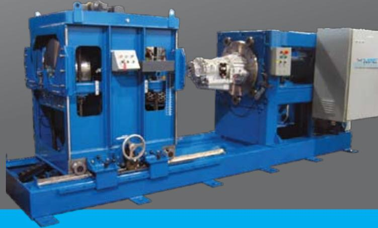
This In-line MD Series system was custom built for Axiom Technologies to test remanufactured transmissions in an end-of-line production environment. The system incorporates many quick-change features to facilitate efficient production testing requirements.
