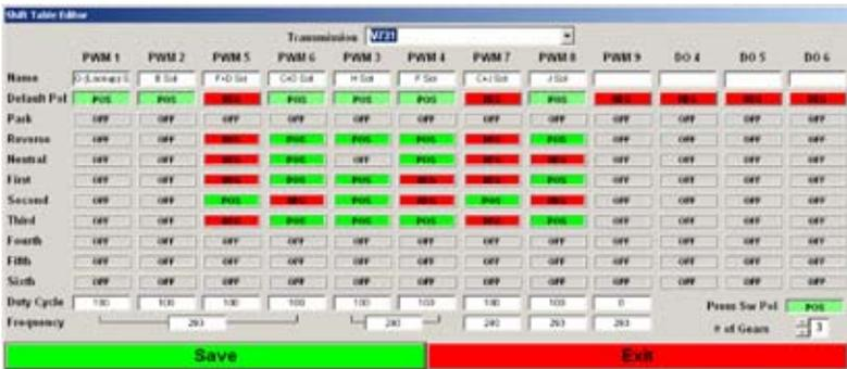
TransTester's Shift Table Editor ensures that you have the flexibility you need to set up a new transmission when the need arises. Using the Shift Table Editor, you have the ability to customize the software to shift any new transmission that may come through your door.
