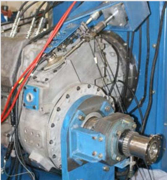
↑ MAE designed, built and delivered this state-of-the-art ED Series cross-drive transmission test bench for Powertrain Plus to test the Abrams M1A1 & M1A2 battle tank's Allison X1100-3B hydraulic steer transmissions. Similar systems have been supplied directly to the US Military to provide state-of-the-art, high throughput final testing various extreme duty battle tank and armored vehicle transmissions.
