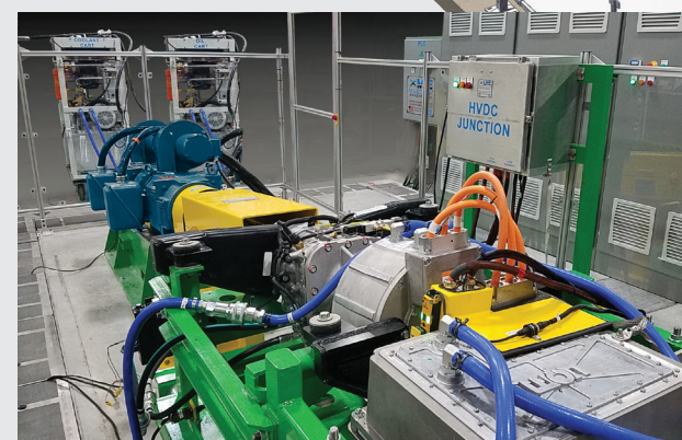
EV Powertrain (Motor, MCU & Gearbox)
