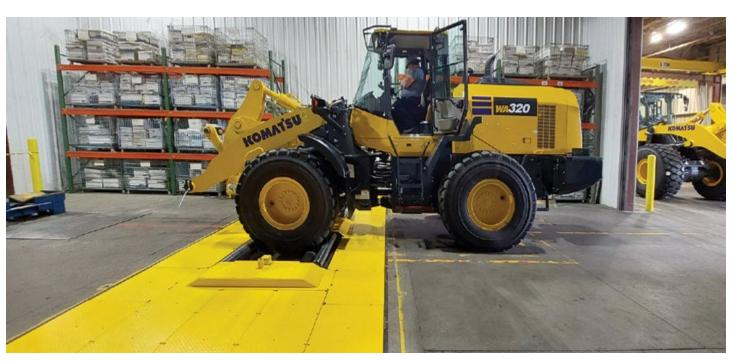
Mustang Advanced Engineering (MAE), an American manufacturer of quality, industry-leading, testing equipment, dynamometers and related products, recently completed the installation of an End-of-Line (EOL) heavy-duty wheel load test stand at Komatsu's Newberry, South Carolina plant.
