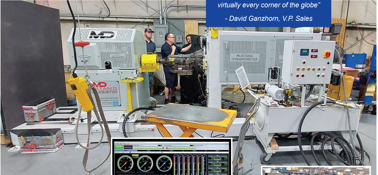
MAE’s new TESTCell™ automation and data acquisition software is used in the operation of the dynamometer
