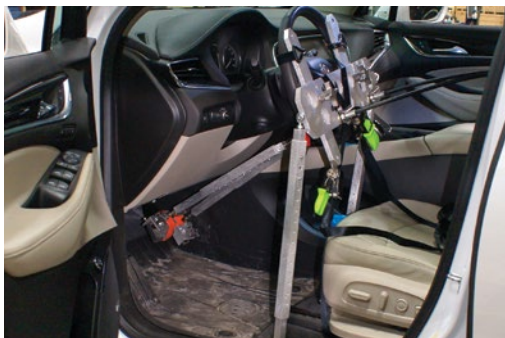
Robotic pedal-throttle actuators for automatic driving
