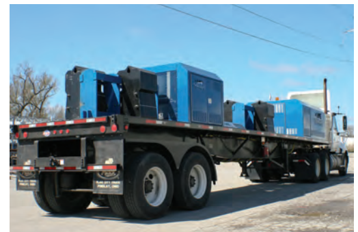
Converted vehicle into a mobile style tow dyno
