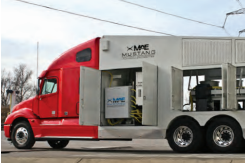
Converted vehicle into a mobile style tow dynamometer
