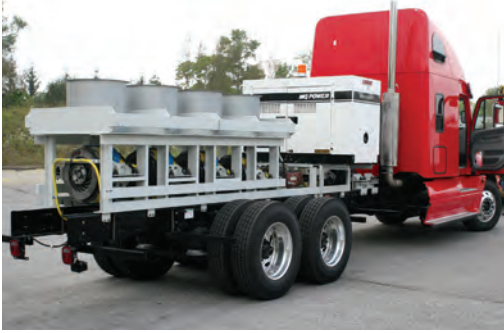
Converted vehicle into a mobile style tow dyno
