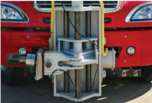
Swing connection for mobile style tow dynamometer
