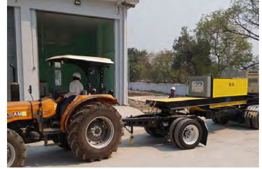
Agricultural MDT-90KN tow dynamometer
