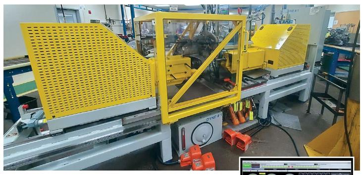
MAE's TESTCell™ data acquisition software is used in the operation of the transmission dynamometers
