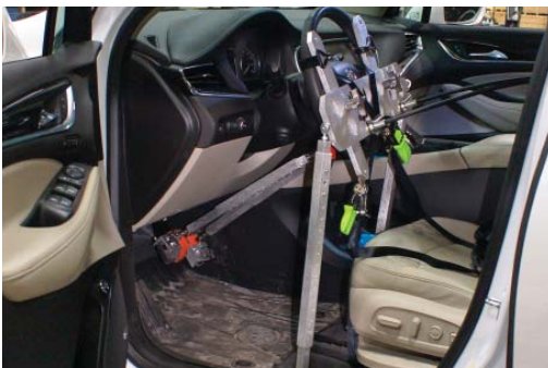
Robotic pedal-throttle actuators for automatic driving
